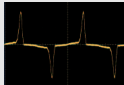
Photo (a) Current waveform of rectified load
